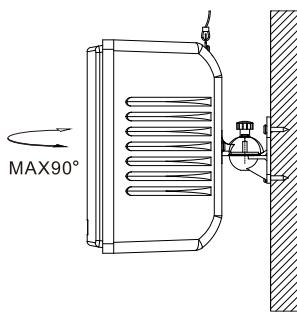
7.If safety strap is required to be installed, please use the KA4\*15 screw to fix it to the speaker as shown below.
